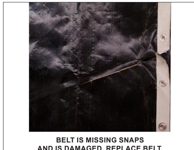
Figure 6. Example of Damaged Belt
