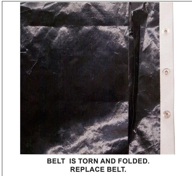
Figure 5. Example of Damaged Belt
