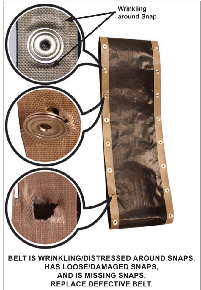
Figure 7. Example of Damaged Belt
